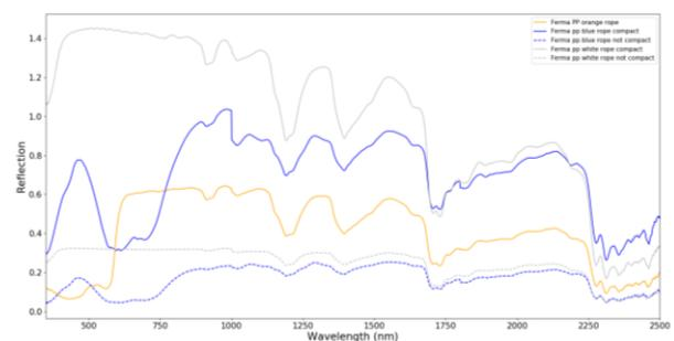
Fig. 1: Spectral reflectance of different PP ropes
