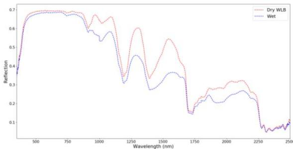
Fig.3: White rope, wet and dry condition
