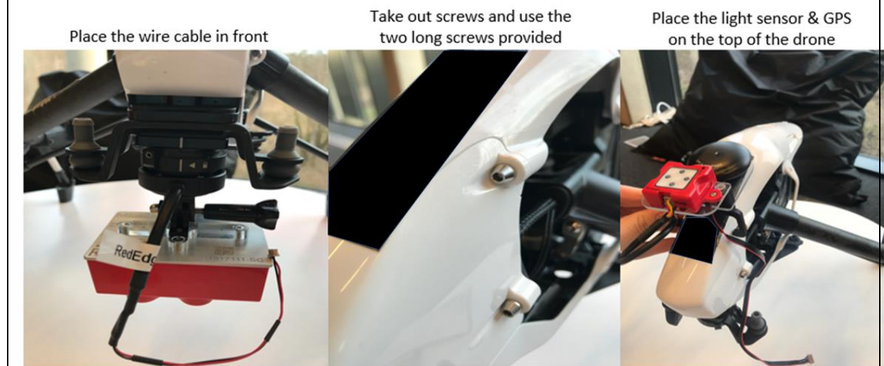
Figure 3: Mounting a MicaSense camera on an Inspire1 drone
