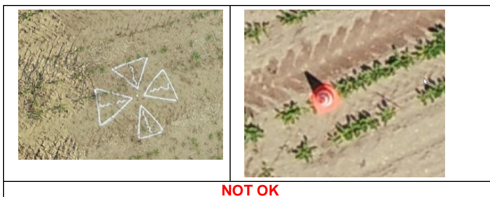
Figure 2: Improper GCP markers
