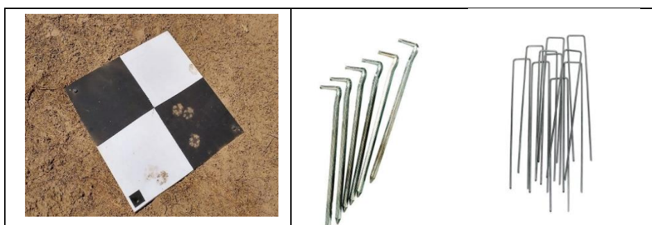
Figure 1: Proper GCP banners and ground pegs
