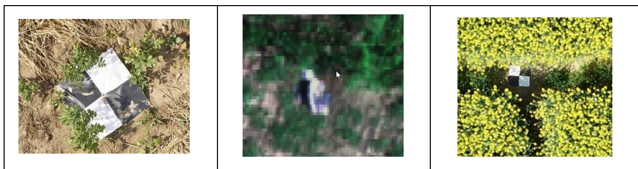
Figure 5: Poor visibility of GCPs
